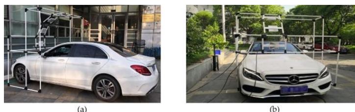
Figure 4. Outdoor static test setup for ERI tag evaluation. (a) Side view of the height-adjustable frame holding four linearly polarized patch antennas; the vehicle is parked at the measurement position and the reader/measurement unit is placed to the side. (b) Front view showing the four antennas arranged to realize incidence angles of 0^\circ , 30^\circ , 60^\circ , and 90^\circ around the tag location on the windshield. Frequency sweeps across 920–925 MHz were performed at each angle under the same static geometry as in the anechoic-chamber tests.
